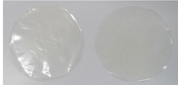
Figure 1. Active biofilms with citralmicroparticles formulated with CS:Sb ratio (1:1.0) and CS:MC ratio (1:0.5), photography taken immediately after of its processing.
