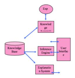
Figure 2.Structure of an Expert System Shell
