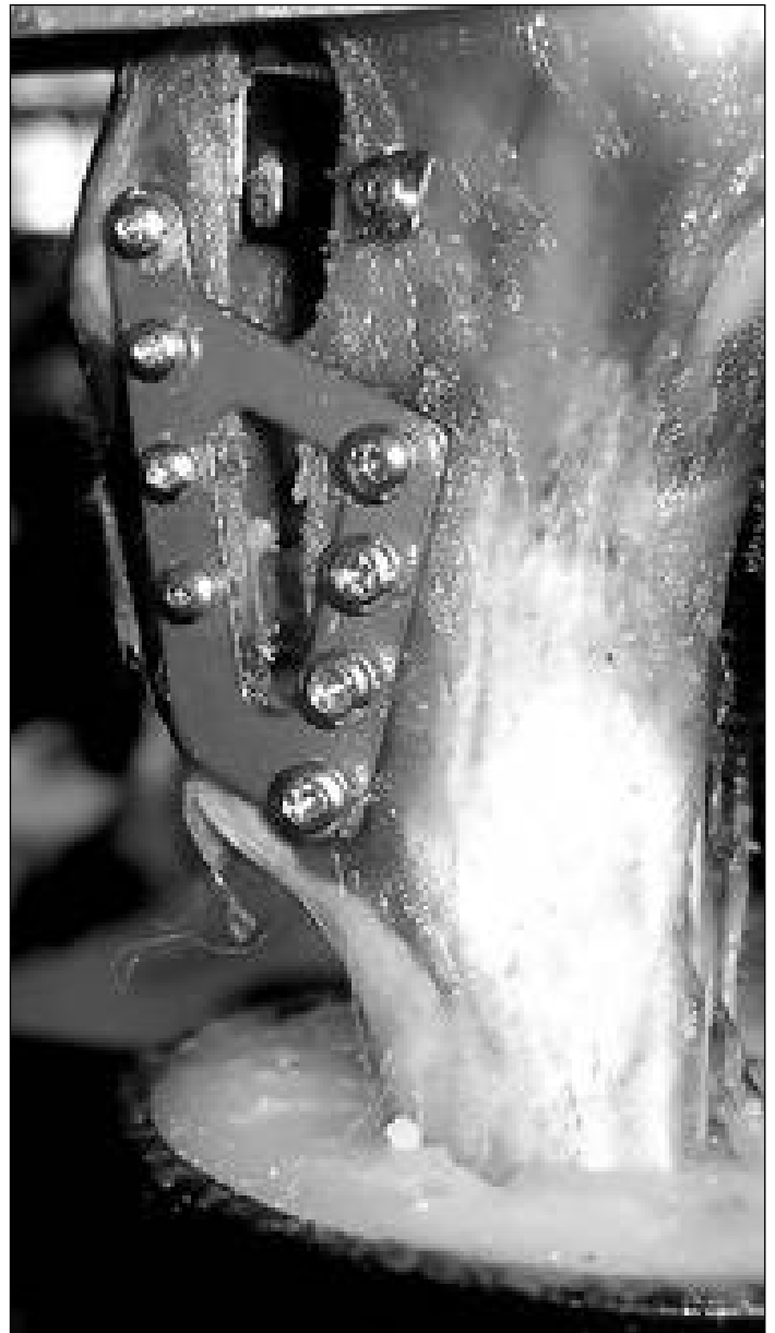
FIGURE 4. POSITIONING OF THE DEVICE ON THE SPECIMEN TO BE TESTED, AND FIXATION WITH SCREWS.
